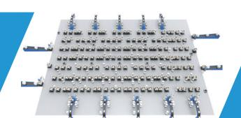
Geek+ robots are driven by innovative AI algorithms to achieve maximum sorting efficiency. Flexible route assignment finds the most effective route in the sorting process, thus reducing the time required. The self-propelled robots automatically carry out fast sorting and bring the loads to the appropriate destination points.
